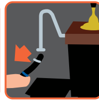
DISCONNECT waste pipe
